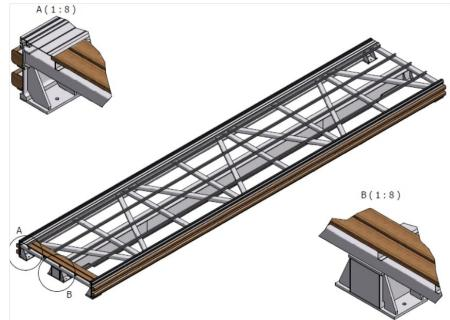
The profiles have a top guide rail and two side rails which allow a slide mounting for mooring cleats and other accessories.
